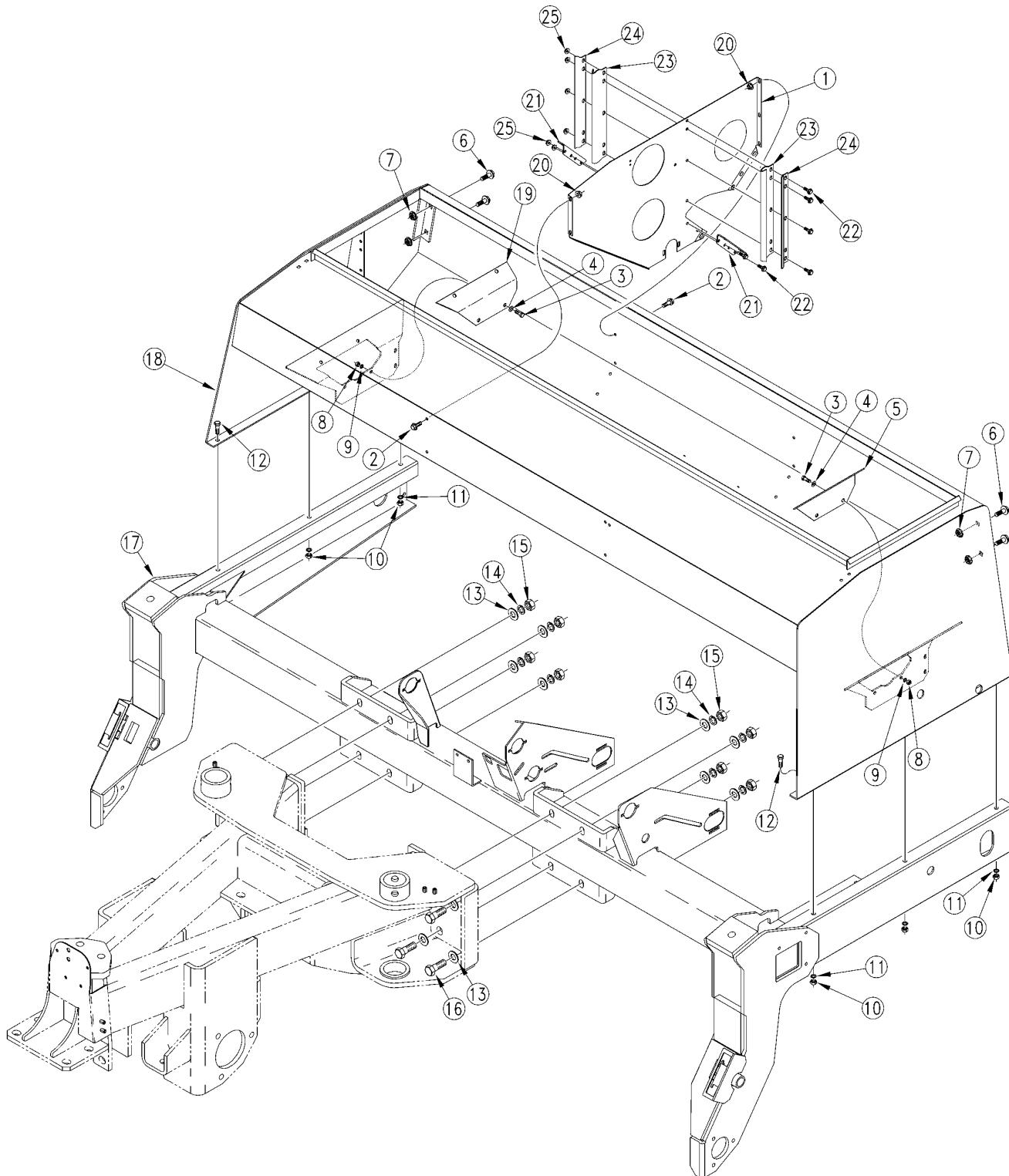
**Center Box And Center Frame To Mainframe Fertilizer**
