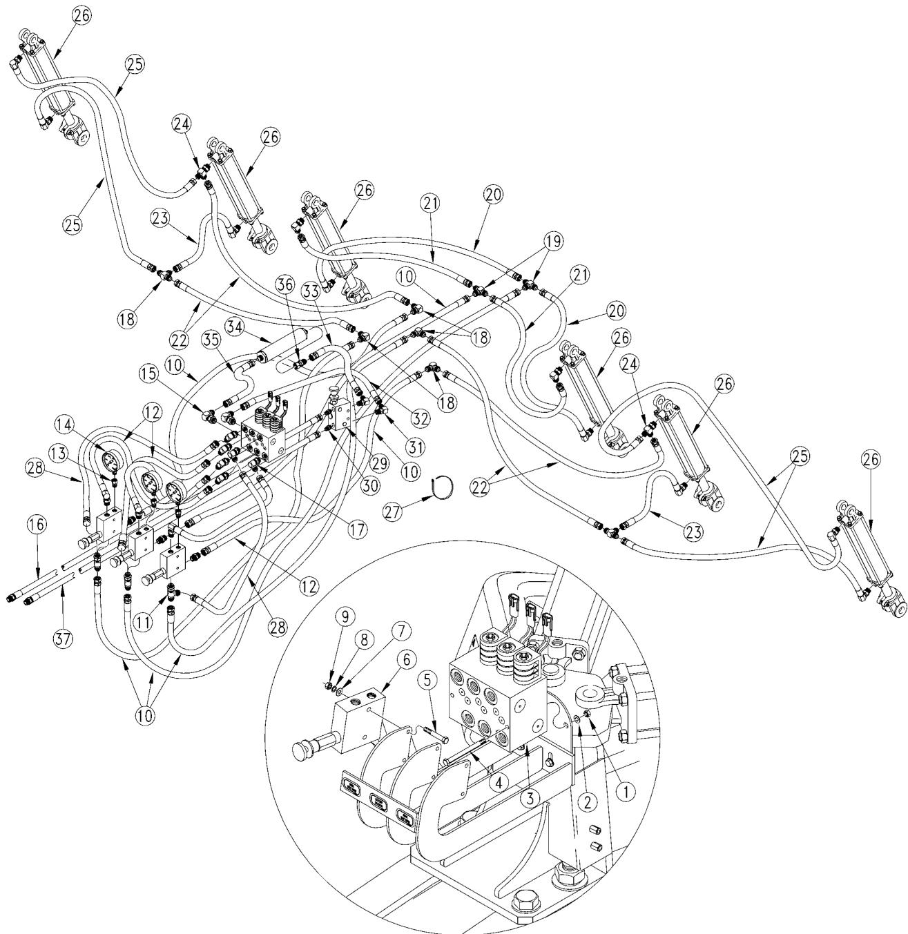
**Opener Down Pressure Hydraulics With Point Row (Option) (S/N S1699-)**
