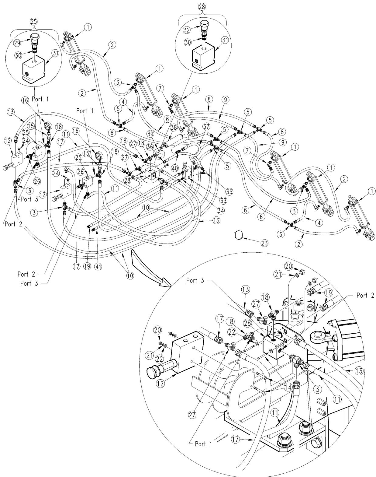
**Opener Down Pressure Hydraulics (Open Center) (S/N S1699-)**
