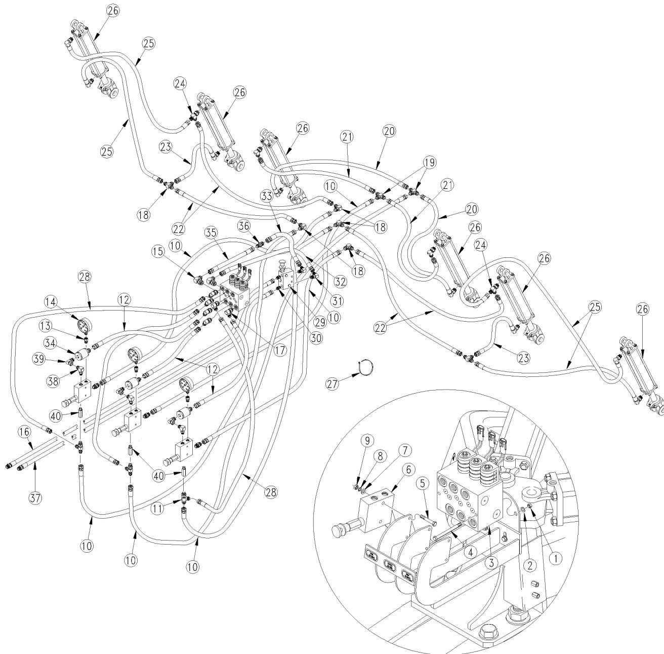
**Opener Down Pressure Hydraulics With Point Row (Option) (S/N S1700+)**
