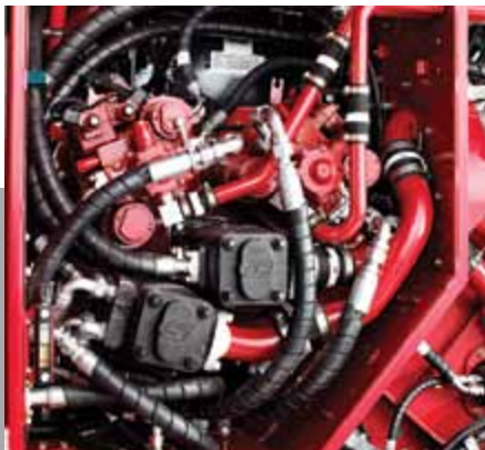
3-stage Parker Pump – greater oil flow to the motors of the chopper.
