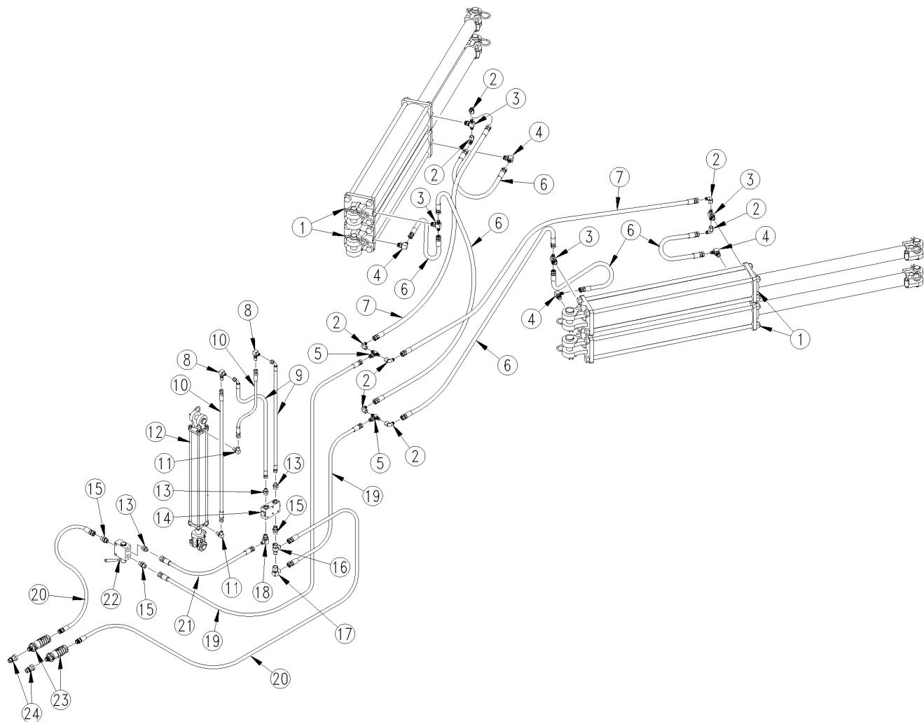
**Fold Hydraulics With Hydraulic Jack (S/N C1288L - C1295L)**
