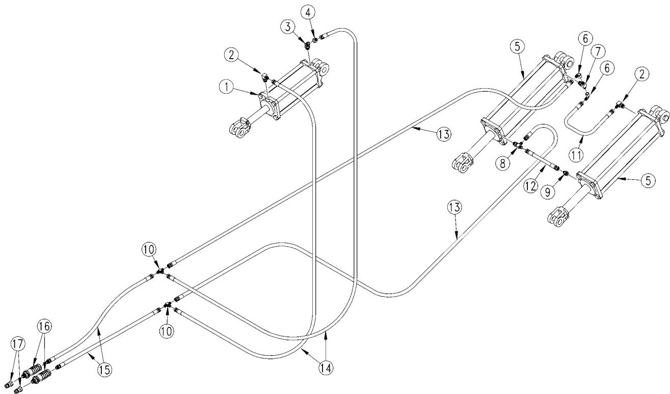
**Transport Axle Hydraulics and Transport Hook Hydraulics**
