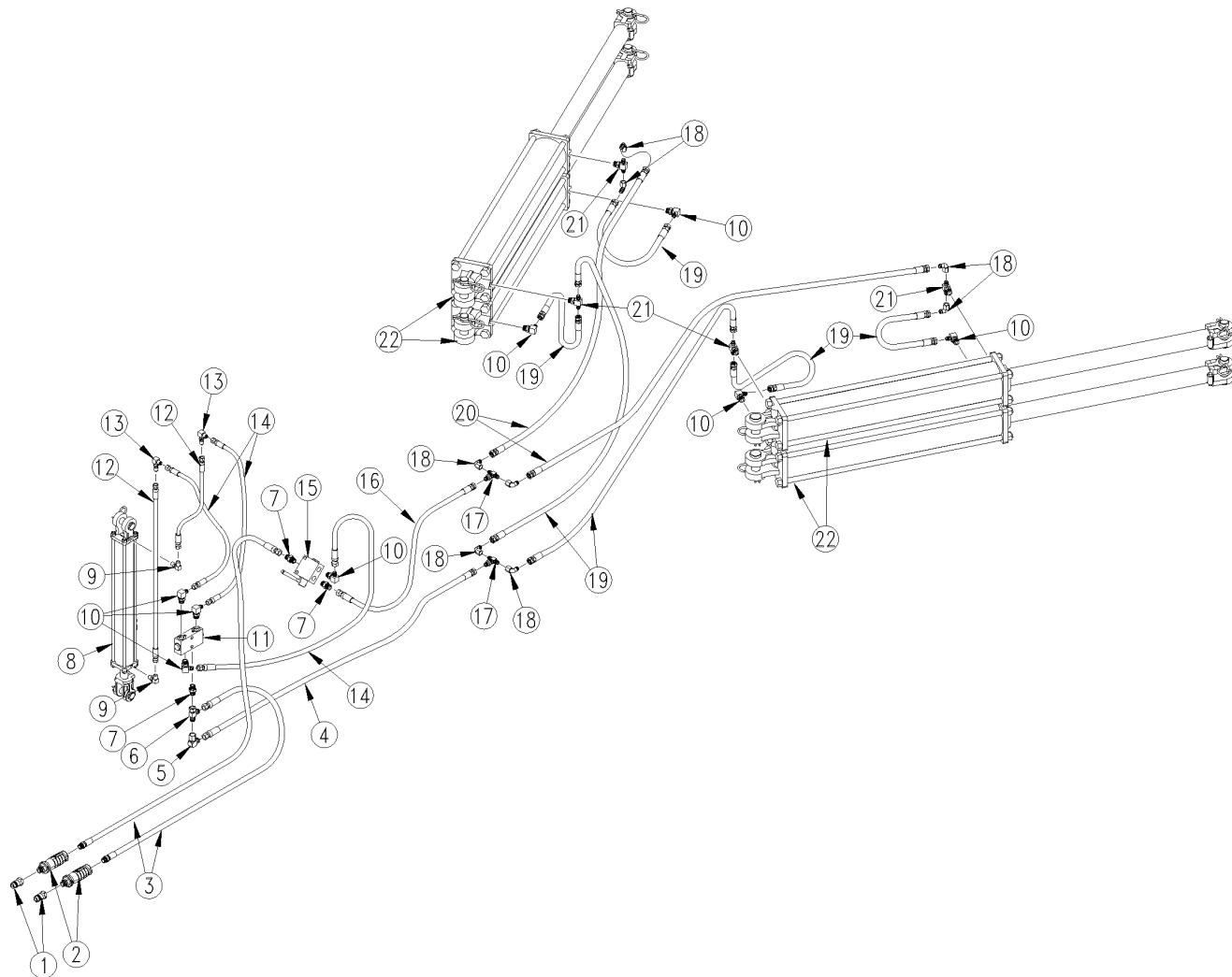
**Fold Hydraulics With Hydraulic Jack (S/N C1296L+)**
