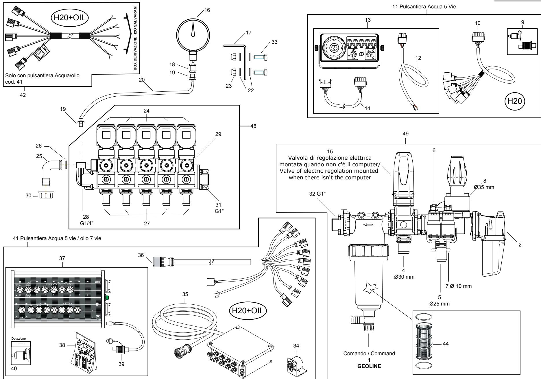
**GCP elettrico Remo 5V trainati+pulsant. / Pressure regulator trailed + control panel**
